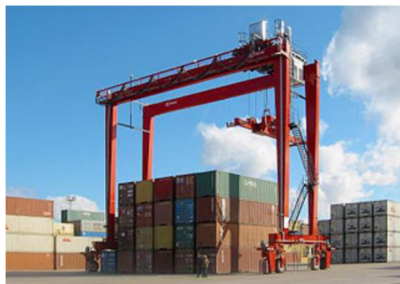
Figura 3. Rubber Tyre Gantry Crane (RTG).
